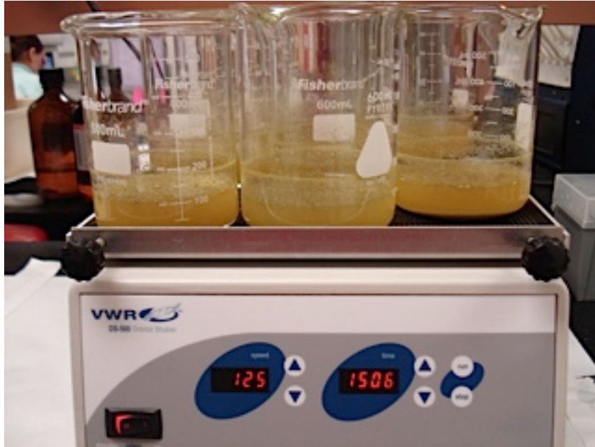
Figure 7. Dry hops mixing on an orbital shaker (photograph by M. Schmick)
