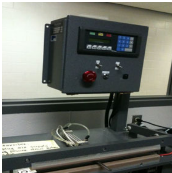
Figure 3. Advanced thermal impulse heat sealing equipment, Mansfield, Texas.
