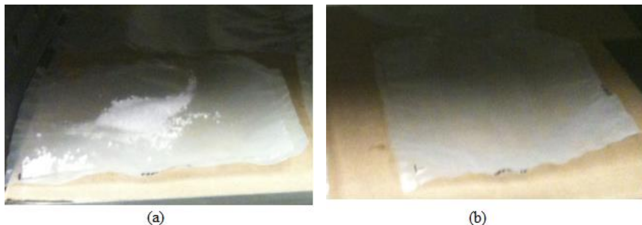
Figure 5. (a) Closed condition with 10 gm desiccant, (b) Control – no desiccant
