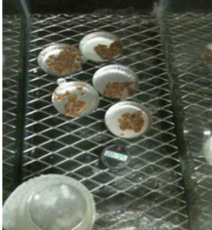
Figure 2. A top view of the samples in a humidity chamber maintained at 60% RH
