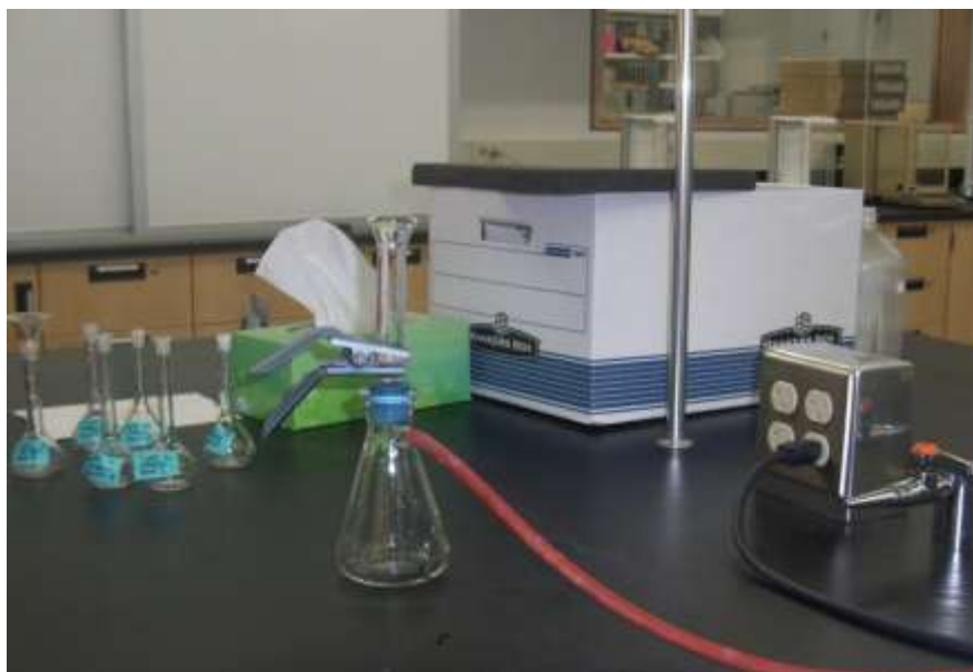
Figure 7. Filtration set up for roots and shoots digested samples
