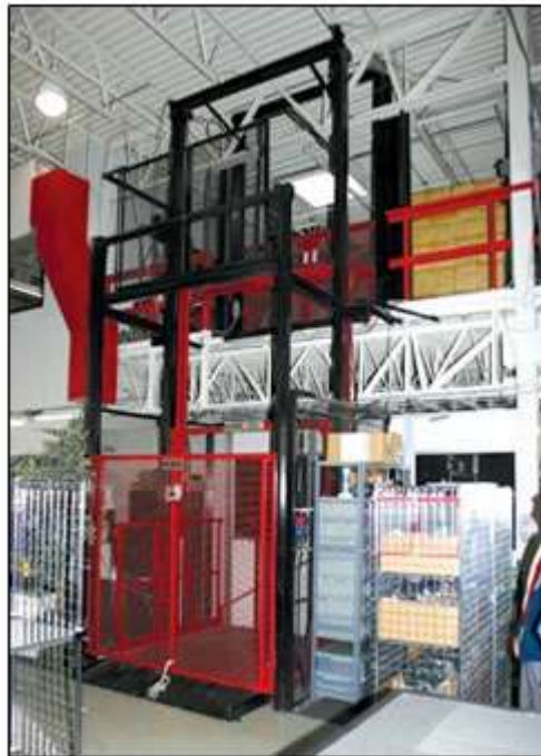
Figure 3. Elevator for Mezzanine System from http://www.alphamaterialhandling.com/mezz_lifts.html
