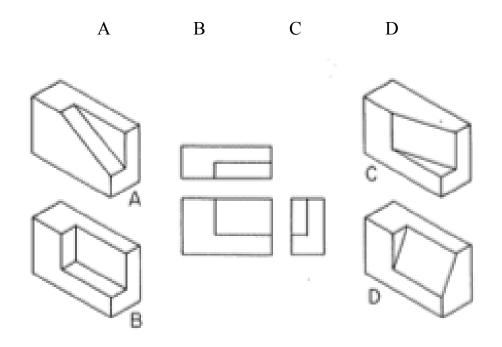
**14.** Circle the rotated object in the left set that is shown in the orthographic projection on the right.
