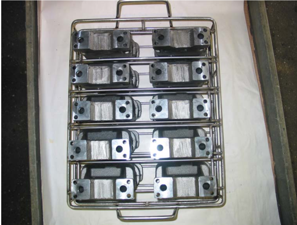
Figure 2: Washing Basket Loaded with Castings
