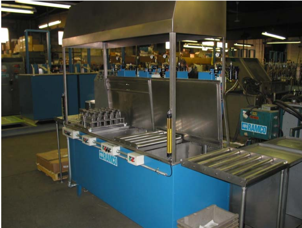
Parts Washer with Lids Open and Parts Basket in Stage 1 Wash
