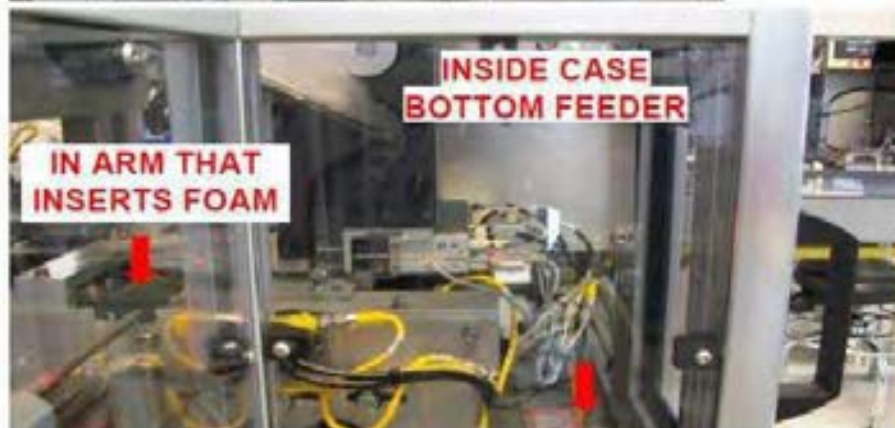
CLOSE UP OF CASE BOTTOM FEEDER TRACK
