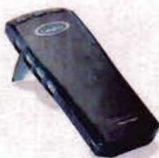
Figure 2: Motion Sensor The motion detector sensor attaches to the LabPro to start and stop time in velocity, acceleration, position, and other motion-type data.
