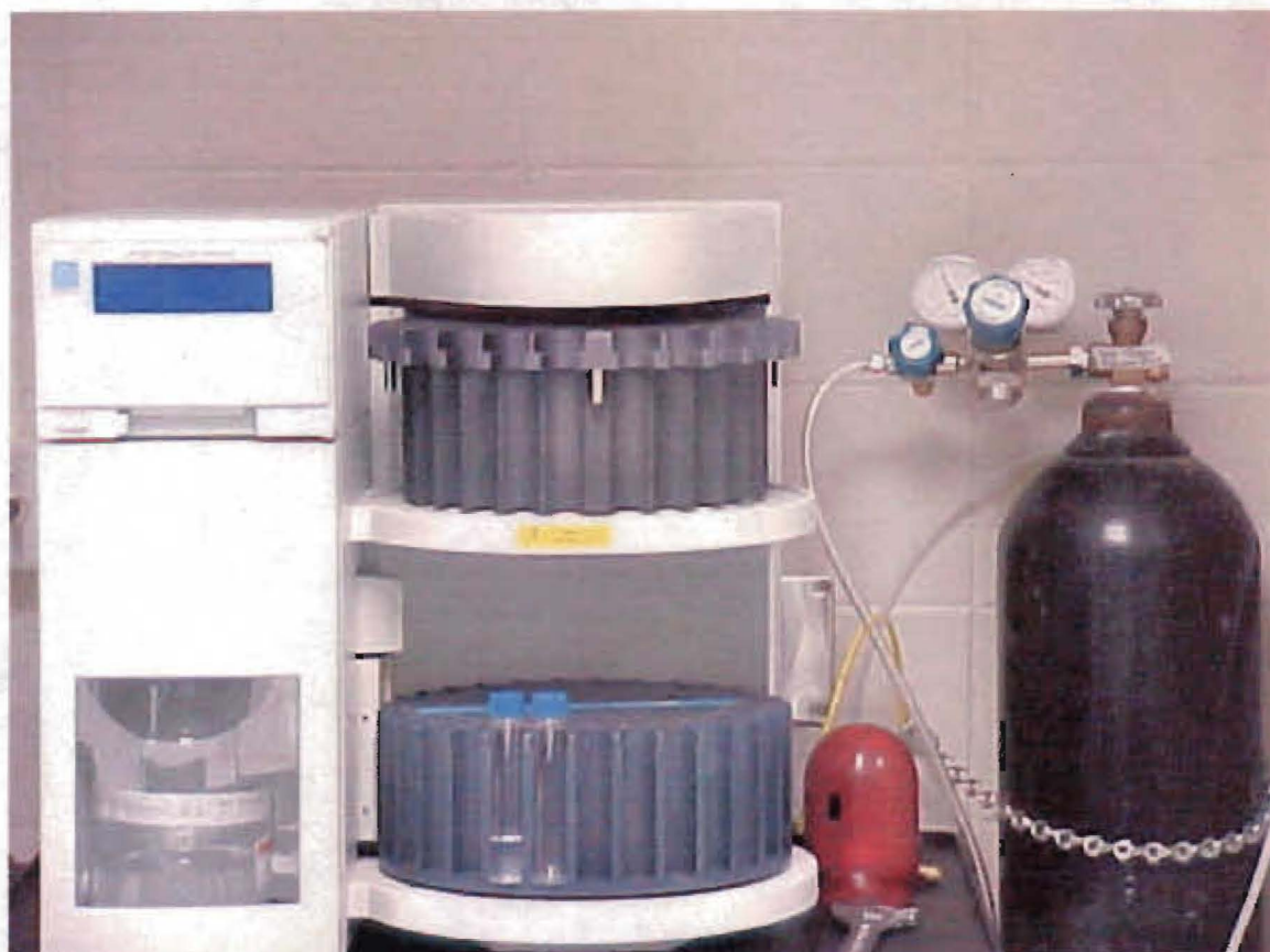
Figure 3: Accelerated solvent extractor used for extracting crude fat for organic milk and cheese
