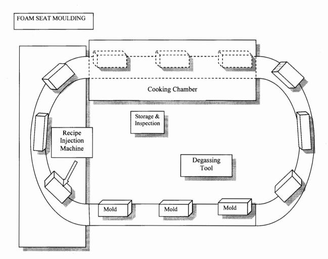
Figure 3) Current State Value Stream of an Injection Molding Process, March 2005
