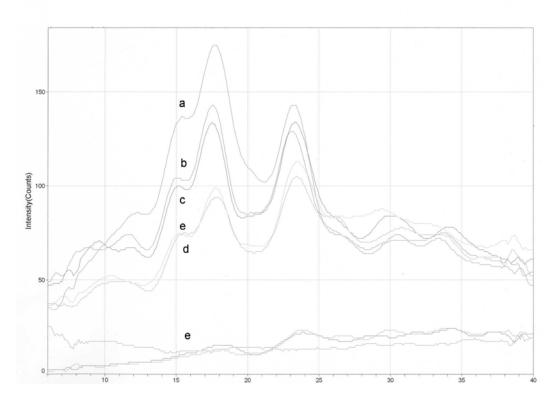
Figure 3. X-ray Diffraction Reading for Unheated Buckwheat Starch Moisture levels: a - 13.2%, b - 26.8%, c - 32.3%, d - 40.0%, e. 44.4% (2)
