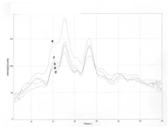
Figure 4. X-ray Diffraction Reading for Heated Buckwheat Starch Moisture levels: a - 13.2%, b - 26.8%, c - 32.3%, d - 40.0%, e. 44.4%
