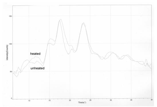
Figure 7. X-ray Diffraction Reading for Unheated and Heated 32.3% Moisture Level Buckwheat Starch
