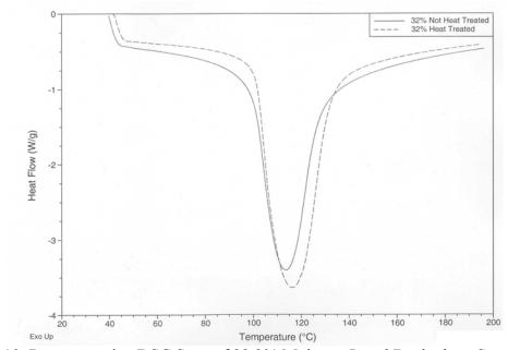
Figure 10. Representative DSC Scan of 32.3% Moisture Level Buckwheat Starch
