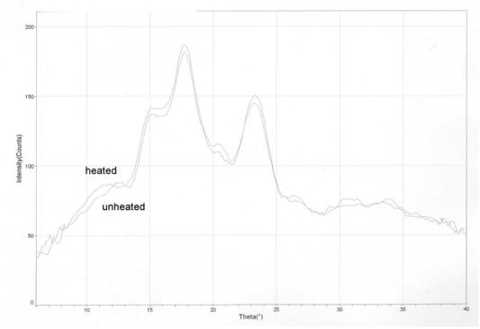
Figure 5. X-ray Diffraction Reading for Unheated and Heated 13.2% Moisture Level Buckwheat Starch
