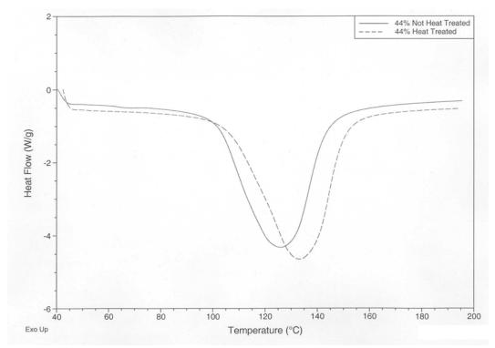
Figure 12. Representative DSC Scan of 44.4% Moisture Level Buckwheat Starch
