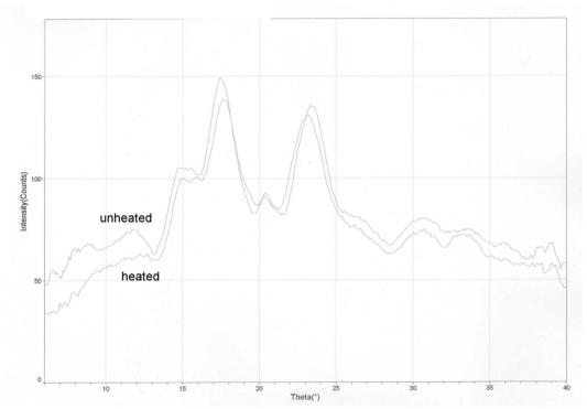
Figure 6. X-ray Diffraction Reading for Unheated and Heated 26.8% Moisture Level Buckwheat Starch
