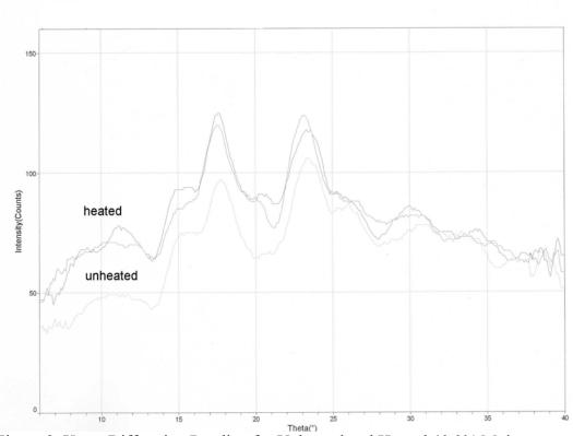
Figure 8. X-ray Diffraction Reading for Unheated and Heated 40.0% Moisture Level Buckwheat Starch
