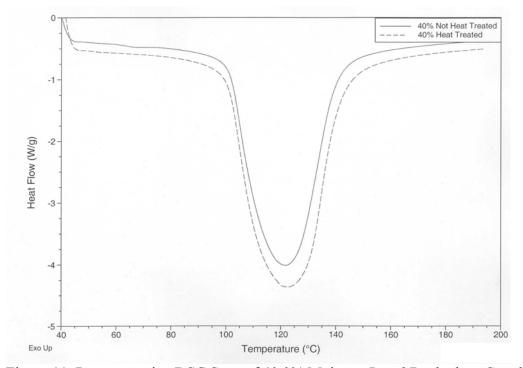
Figure 11. Representative DSC Scan of 40.0% Moisture Level Buckwheat Starch
