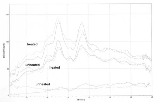
Figure 9. X-ray Diffraction Reading for Unheated and Heated 44.4% Moisture Level Buckwheat Starch
