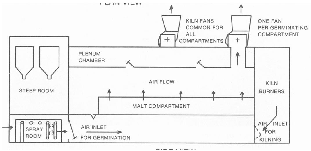
Figure 1. Diagram of typical malthouse.
