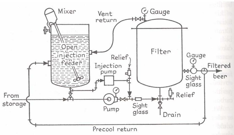
Figure 4. Diagram of a typical wire mesh kieselguhr filter
