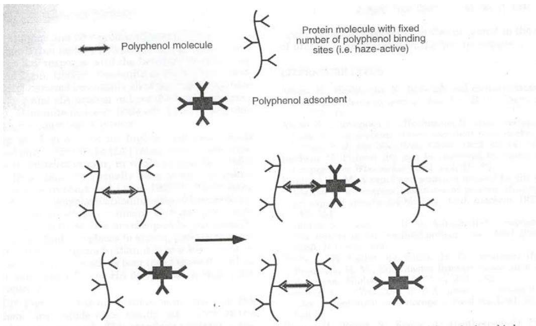
Figure 7. PVPP adsorption of beer haze-active polyphenols: PVPP is specific for haze-active polyphenols.
