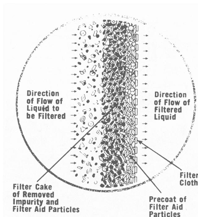
Figure 5. Filter Septum with the pre-coat and filter cake.
