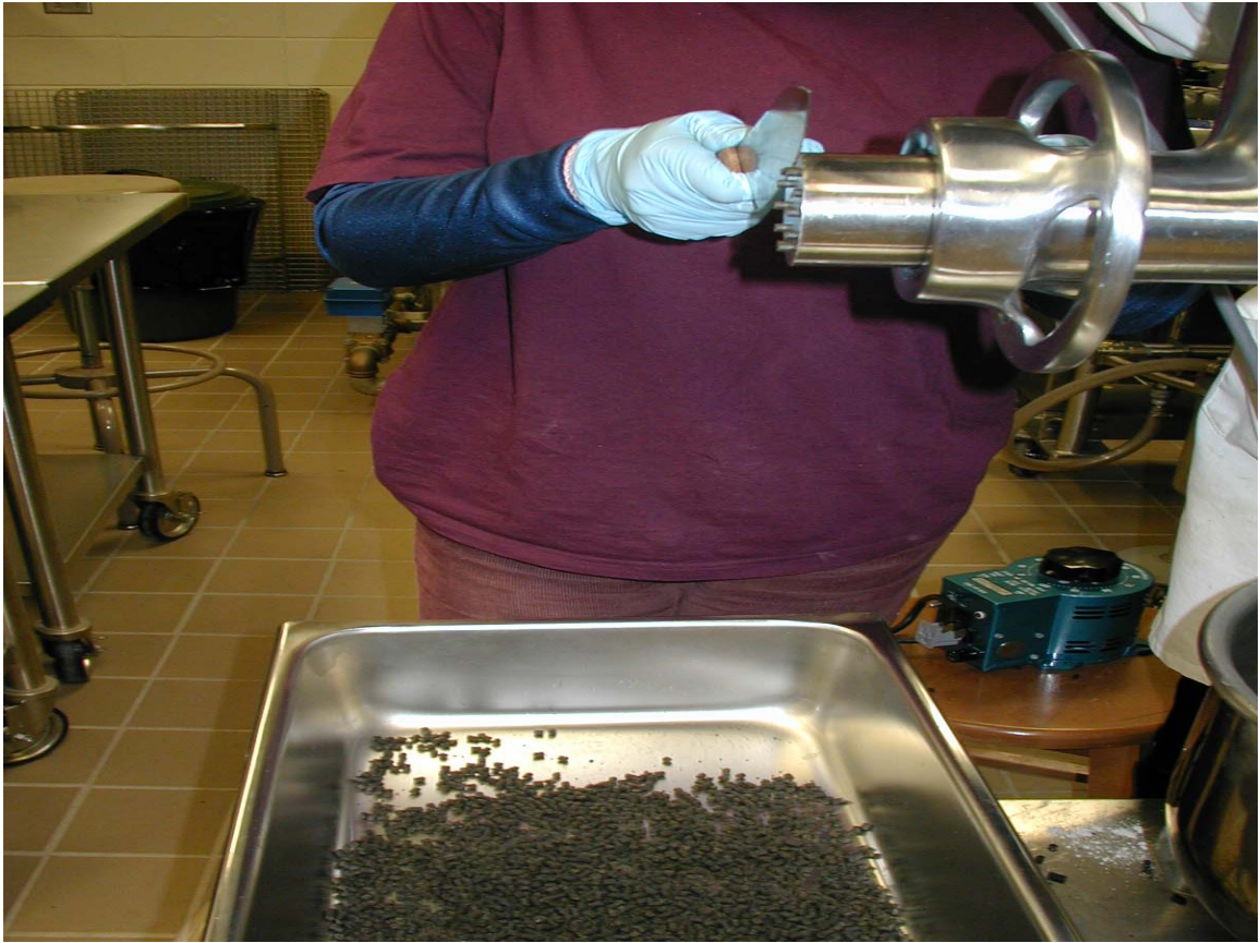
Figure 10. Flow through the die and fish pellets
