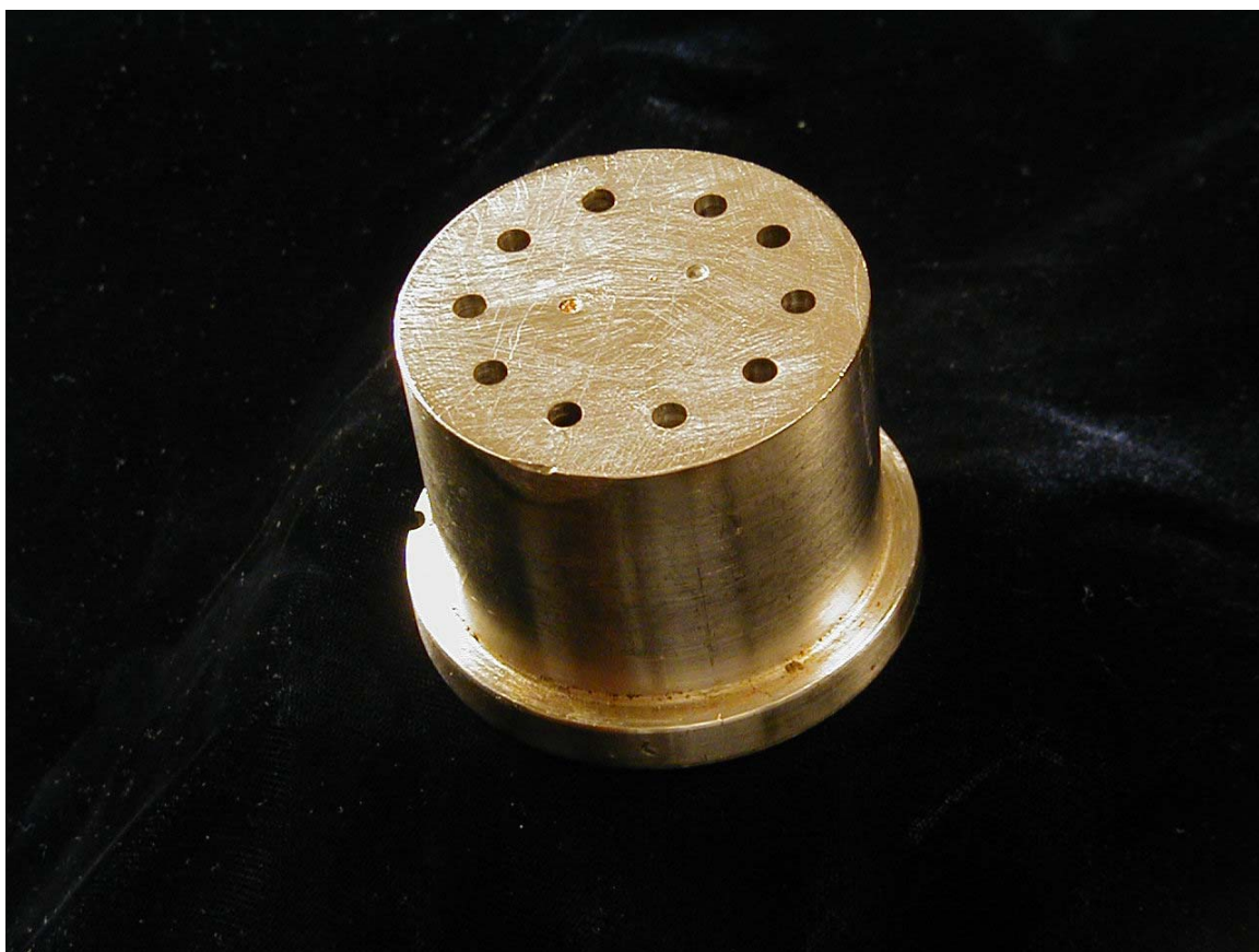
Figure 8. Die used for extrusion of the of the fish pellets
