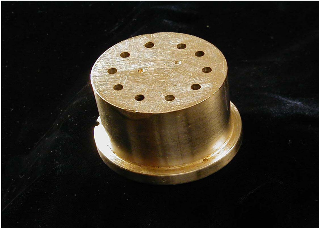
Figure 6. Die used for extrusion of the fish pellets
