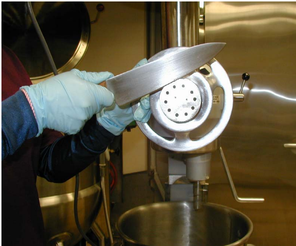
Figure 9. Die attached to the Hobart extrusion attachment
