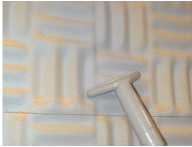
Figure 3.15. Cleaning of SONEX was performed using a standard vacuum and attachment.
