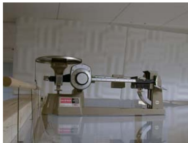
Figure 3.6. SONEX panel weighing system consisting of scale and cross member that was attached to four strings affixed to removable hooks.
