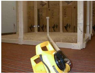
Figure 3.13. A standard single speed leaf blower introduced wood particulate into the chamber by means of a PVC pipe delivery apparatus.
