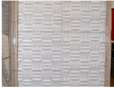
Figure 3.8. SONEX panels pressed to the wall of the chamber by nylon string.
