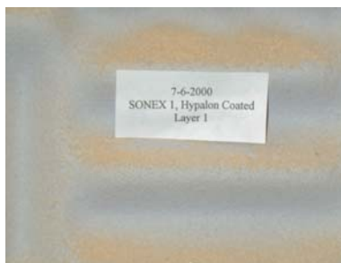
Figure 4.2. Photograph demonstrating the amount of wood particulate on the SONEX Hypalon coated acoustical panels during layer 1 deposition.
