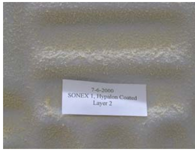
Figure 4.3. Photograph of the particulate level on Hypalon coated SONEX for particulate layer 2.
