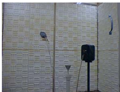
Figure 3.9. Stereo speaker placement directed to the back right corner of the chamber 0.91 meter high.
