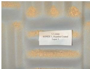
Figure 4.4. Close up photograph of particulate layer 3 on Hypalon coated SONEX.
