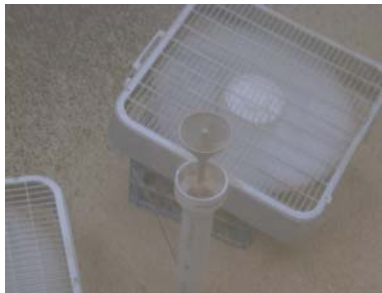
Figure 3.14. A funnel and household box fans were used to facilitate dispersal of wood particulate within the chamber.
