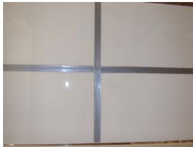
Figure 3.5. Back of four SONEX panels trimmed, glued and taped together.
